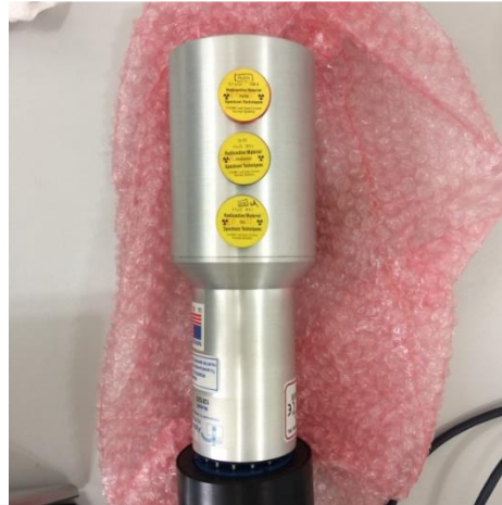
Figure 03: Photo of Gamma ray spectrometer in contact with radioactive sources Cs-137, Sr-90 and Po-210.
